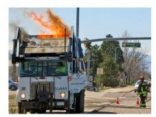
It is especially risky when Li-ion batteries are mistakenly put into a recycling bin and end up bouncing around in the back of a dry recycling truck. Pressure or heat (in the summer months our trucks can get quite hot) can cause them to spark, setting off a chain reaction which spells disaster when that battery is in the back of a full recycling truck, surrounded by dry paper and cardboard. In fact, Li-ion Batteries are one of the leading causes of recycling truck fires.
