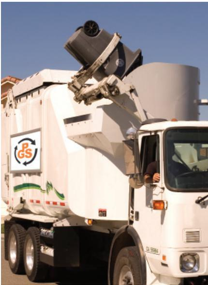
When our automated service trucks come to your home the mechanized arm reaches out and grasps your cart, lifts it up high in the air and dumps it into the truck receiver.
